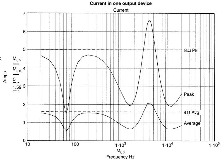
Peak power would appear to be the critical quantity. Power device ratings often allow the power and second-breakdown limits (and sometimes the bondwire current limit also) to be exceeded for brief periods. If you attempt to exploit these areas in an audio application, you are living very dangerously, as the longest excursion specified is usually 5 msec, and a half-cycle at 20 Hz lasts for 25 msec.
