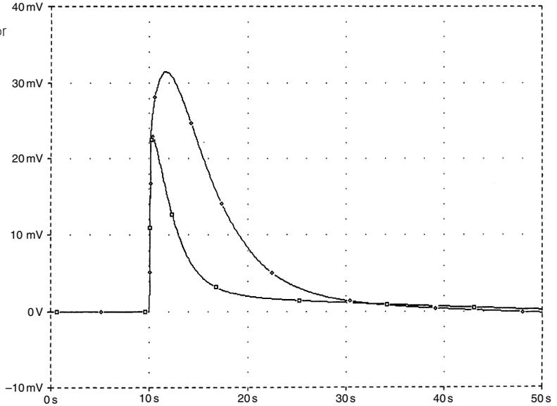
If a thermal pad of standard material is once more used between the sensor and the TO3 top, the optimal  $V_{bias}$  coefficient for minimum error over the first 40 sec proves  $-2.8\text{ mV}/^\circ\text{C}$ , which is usefully less than  $-4.5$ . The resulting 30-sec IAE is  $102\text{ mV}\cdot\text{sec}$ , more than a two times improvement; see the lower trace in Figure 13.16, for comparison with the semi-insulator method described above.
