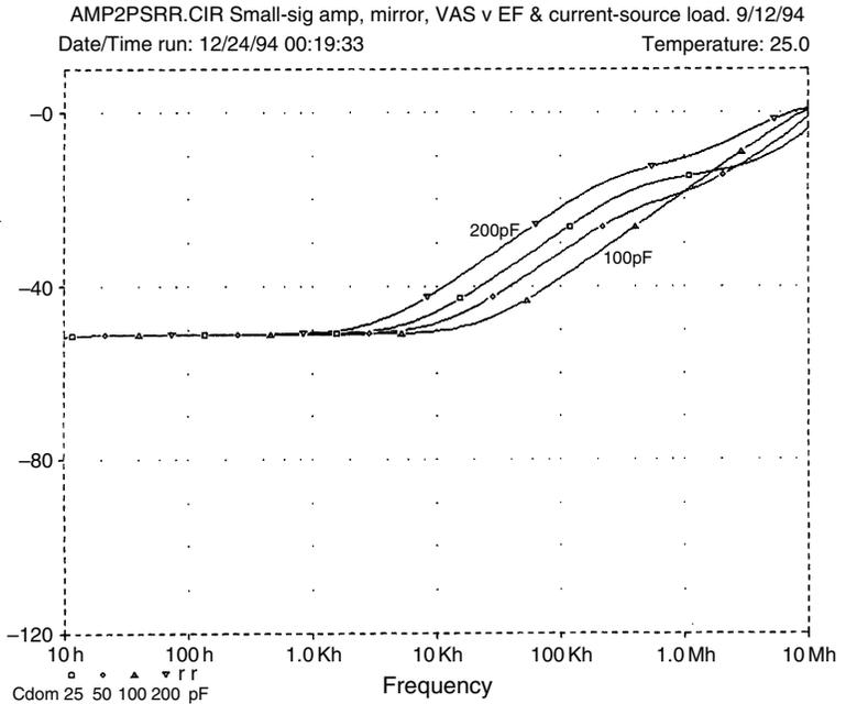
i.e., there is an optimum value for  $C_{dom}$  at about 100 pF, indicating some sort of cancellation effect. (In the  $V+$  case, the value of  $C_{dom}$  made very little difference.)
