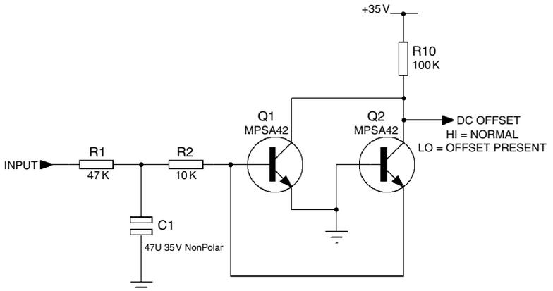
This makes the two thresholds very asymmetrical. When the detector is driven from a single-pole RC filter with  $R1 = 47\text{K}$ , the positive threshold is  $+1.05\text{V}$  but the negative threshold is  $-5.5\text{V}$ . To reduce this asymmetry  $R1$  needs to be kept low, which leads to inconveniently large values of  $C1$ .
