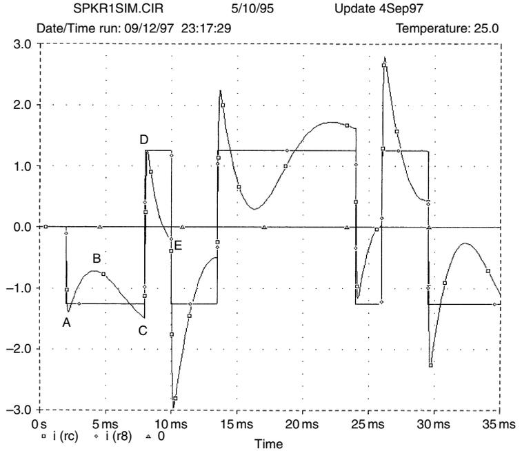
peak goes much lower to 2.96 amps, 2.4 times greater than that drawn by the  $8\ \Omega$  resistor. I call this the Current Timing Factor, or CTF.
