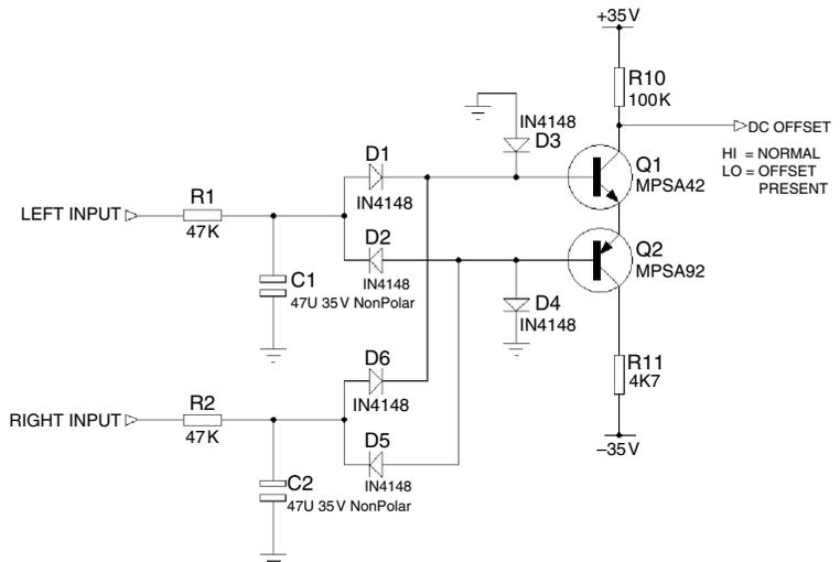
Having paid for a DC protection relay, it seems only sensible to use it for system muting as well, to prevent thuds and bangs from the upstream parts of the audio system from reaching the speakers at power-up and power down. Most power amplifiers, being dual-rail (i.e., DC-coupled) do not generate enormous thumps themselves, but they cannot be guaranteed to be completely silent, and will probably produce an audible turn-on thud.
