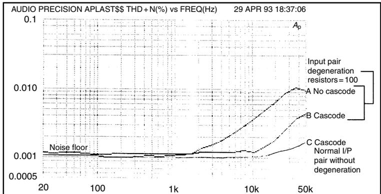
Using a cascode transistor also allows the use of a high-beta transistor for the VAS; these typically have a limited  $V_{ce0}$  that cannot withstand the high rail voltages of a high-power amplifier. There is a small loss of available voltage swing, but only about 300 mV, which is usually tolerable. Experiment shows that there is nothing to be gained by cascoding the current-source collector load.
