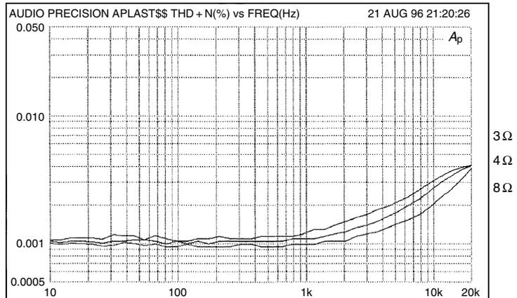
3281/1302 devices will give 50W into 3 Ω for THD of 0.006% (10 kHz), see Figure 5.22. Two pairs of 3281/1302 reduce the distortion to 0.003% (10 kHz) as in Figure 5.23. This is an excellent result for such simple circuitry, and may well be a record for 3 Ω linearity.
