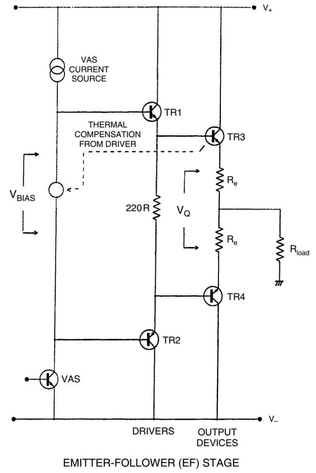
and reasonable. In terms of total  $V_{bias}$ , the EF needs  $2.93\text{ V} \pm 100\text{ mV}$ , and the CFP  $1.30\text{ V} \pm 10\text{ mV}$ .  $V_{bias}$  must be higher in the EF as four  $V_{be}$ 's are subtracted from it to get  $V_q$ , while in the CFP only two driver  $V_{be}$ 's are subtracted.
