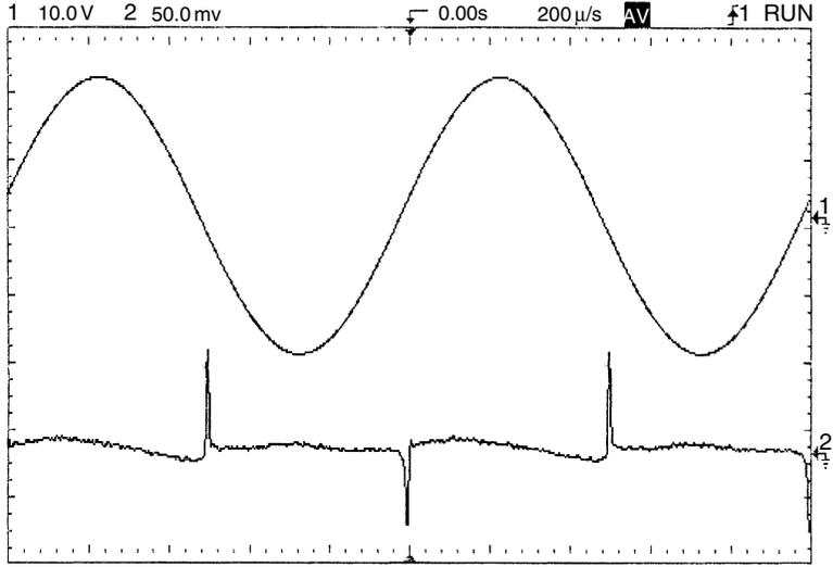
depends strongly on measurement bandwidth. Their presence warns immediately of underbiasing and avoidable crossover distortion.
