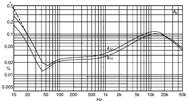
It seems pretty clear that the steep rise here is due to thermal distortion, in the form of feedback from the power output stage to earlier parts of the amplifier – probably the input stage. As would be expected, the effect is greater with a heavier load which causes more heating; in fact halving the load doubles the THD reading below the 40 Hz notch.
