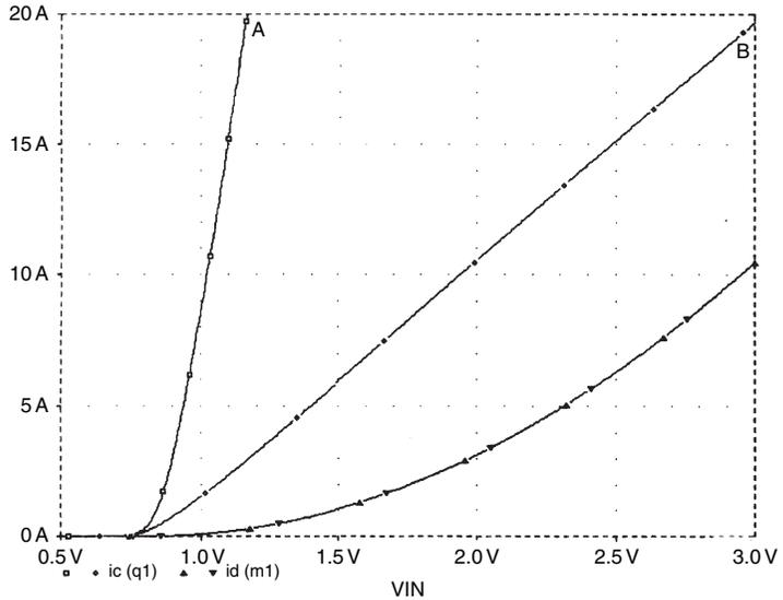
Because of the curved nature of the FET  $I_d$  plot, it is not possible to pick an  $R_e$  value that allows very close gm equivalence;  $R_e = 0.1 \Omega$  was chosen as a reasonable approximation; see Curve B. However, the important point is that I think no-one could argue that the FET  $I_d$  characteristic is more linear than Curve B.
