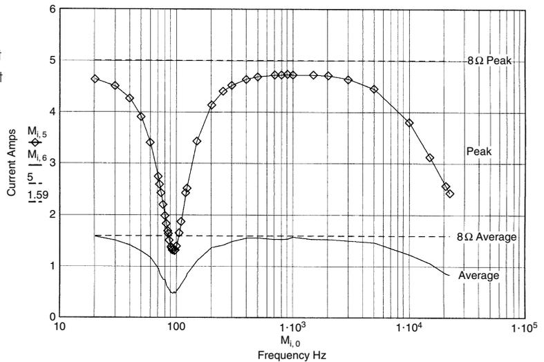
that for an  $8\ \Omega$  resistor (shown dotted) around the actual resonance peak, where it drops quickly to a quarter of the resistive case.
