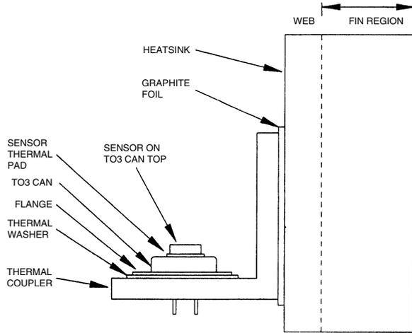
many designs. Dissipation equivalent to  $100\text{W}/8\Omega$  was suddenly initiated, and the temperature of the various parts monitored with thermocouples. The graph clearly shows that the top of the TO3 responds much faster, and with a larger temperature change, though after the first two minutes the temperatures are all increasing at the same rate. The whole assembly took more than an hour to asymptote to thermal equilibrium.
