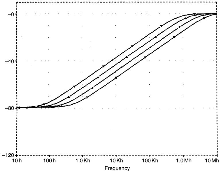
Table 8.2 shows how reducing global NFB by decreasing the value of RNFB degraded ripple rejection in a real amplifier.
