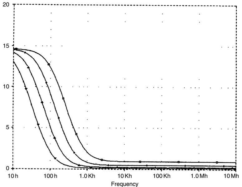
There is an extra complication here; the TR12/TR4 combination actually shows *gain* from V<sub>-</sub> to the output at low frequencies; this is due to Early effect, mostly in TR12. If TR12 was omitted the LF open-loop gain drops to about -6 dB.
