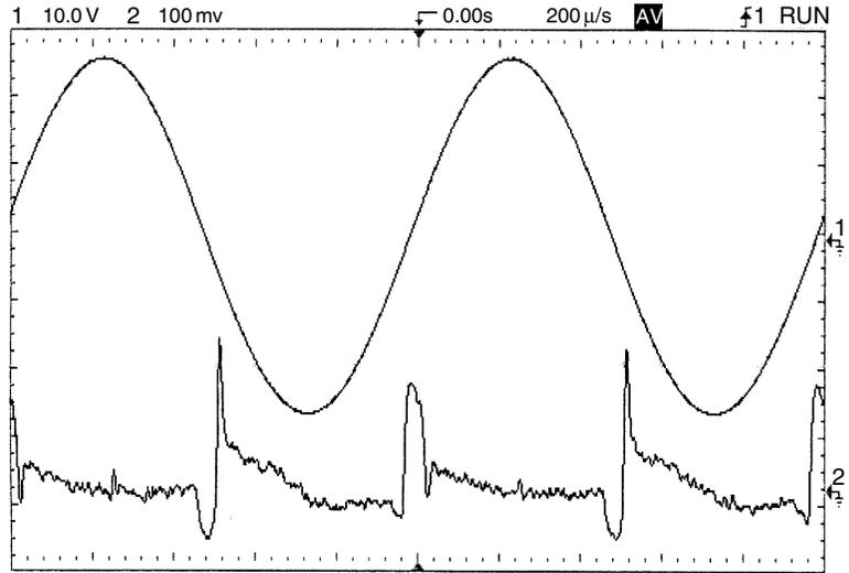
is illustrated in Figure 5.36, which is Figure 5.35 rerun with a 500 kHz bandwidth. The distortion products now look much more jagged.
