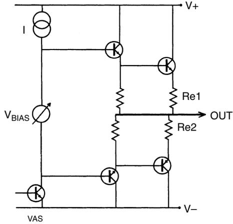
not very practical for discrete power amplifiers; first, in the absence of the very tight thermal coupling between the four junctions that exists in an IC, the quiescent-current stability will be atrocious, with thermal runaway and spontaneous combustion a near-certainty. Second, the output device bulk emitter resistance will probably give enough voltage drop to turn the other device off anyway, when current flows. The need for drivers, with their extra junction-drops, also complicates things.
