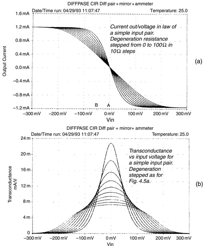
is reduced, but the curve made flatter and linear over a wider operating range. Simply adding emitter degeneration markedly improves the linearity of the input stage, but the noise performance is slightly worsened, and of course the overall amplifier feedback factor has been reduced, for as previously shown, the vitally-important HF closed-loop gain is determined solely by the input transconductance and the value of the dominant-pole capacitor.
