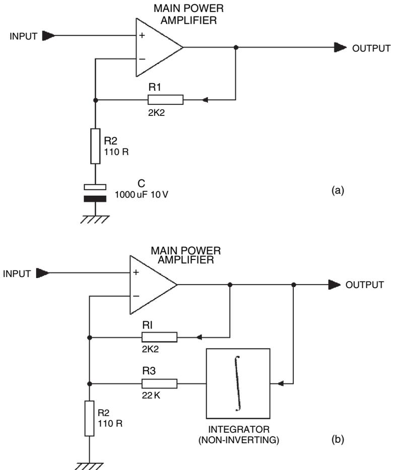
point is that the integrator block must be non-inverting for the servo feedback to be in the correct phase. The standard shunt-feedback integrator is of course inverting, so something needs to be done about that. Several non-inverting integrators are examined below.
