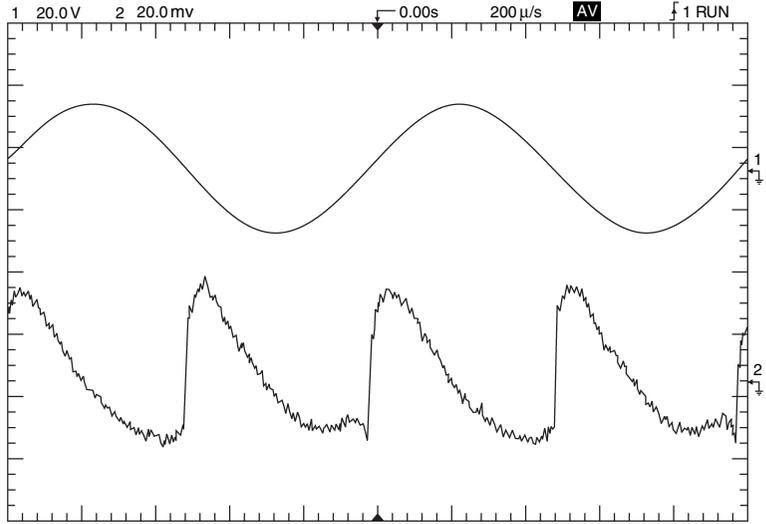
A Distortion 6 residual is displayed in Figure 6.8. The V-supply rail was routed parallel to the negative-feedback line to produce this diagram. THD is more than doubled, but is still relatively low at 0.0021%. 64-times averaging is used. Distortion 6 is easily identified if the DC supply cables are movable, for altering their run will strongly affect the quantity generated.
