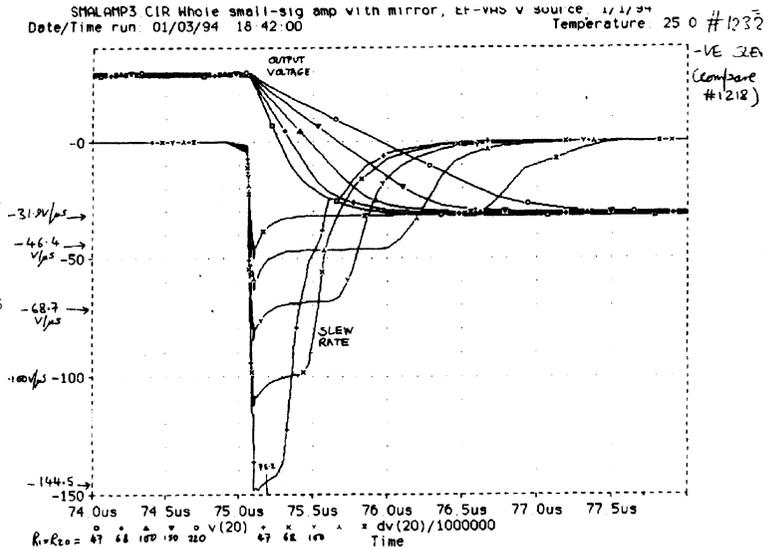
Several points need to be made about these plots; first, the slew-rates shown for the lower  $R_4$ , 23 values are not obtainable in the real amplifier with output stage, for reasons that will emerge. Note that almost imperceptible wobbles in the output voltage put large spikes on the plot of the slew-rate, and it is unlikely that these are being simulated accurately, if only because circuit strays are neglected. To get valid slew-rates, read the flat portions of the differential plots.
