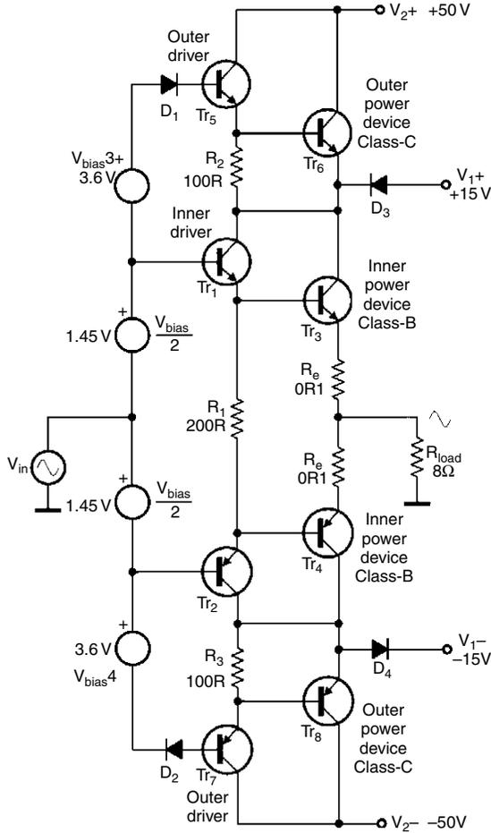
inner power devices work in Class-B it is their temperature which must be tracked to maintain quiescent conditions. Power from the lower supply is drawn through D3 and D4, often called the commutating diodes, to emphasise their rail-switching action. The word ‘commutation’ avoids confusion with the usual Class-B crossover at zero volts. I have called the level at which rail-switching occurs the transition level.
