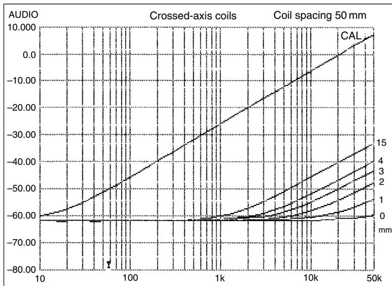
spacing is unlikely to be less than 50 mm unless the output components have been deliberately grouped together. As with capacitive crosstalk, physical distance is cheaper than anything else, and if the results are not good enough, use more of it. In this case the overall crosstalk at 20 kHz will be  $54 + 38 = -92$  dB total, which is probably already well below other forms of interchannel crosstalk. A quick quarter-turn of the coil improves this to at least  $-114$  dB. It should do.
