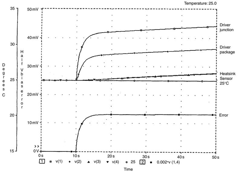
We might expect the CFP delay errors to be much shorter than in the EF; however, simulation with a heat step-input suitably scaled down to 0.5 W (Figure 13.13) shows changes in temperature error V(1)–V(4) that appear rather paradoxical; the error reaches 5° in 1.8 seconds, levelling out at 6.5° after about 6 sec. This is markedly slower than the EF case, and gives a total bias error of +13 mV, which after doubling to +26 mV is well outside the CFP error band of ±10 mV.
