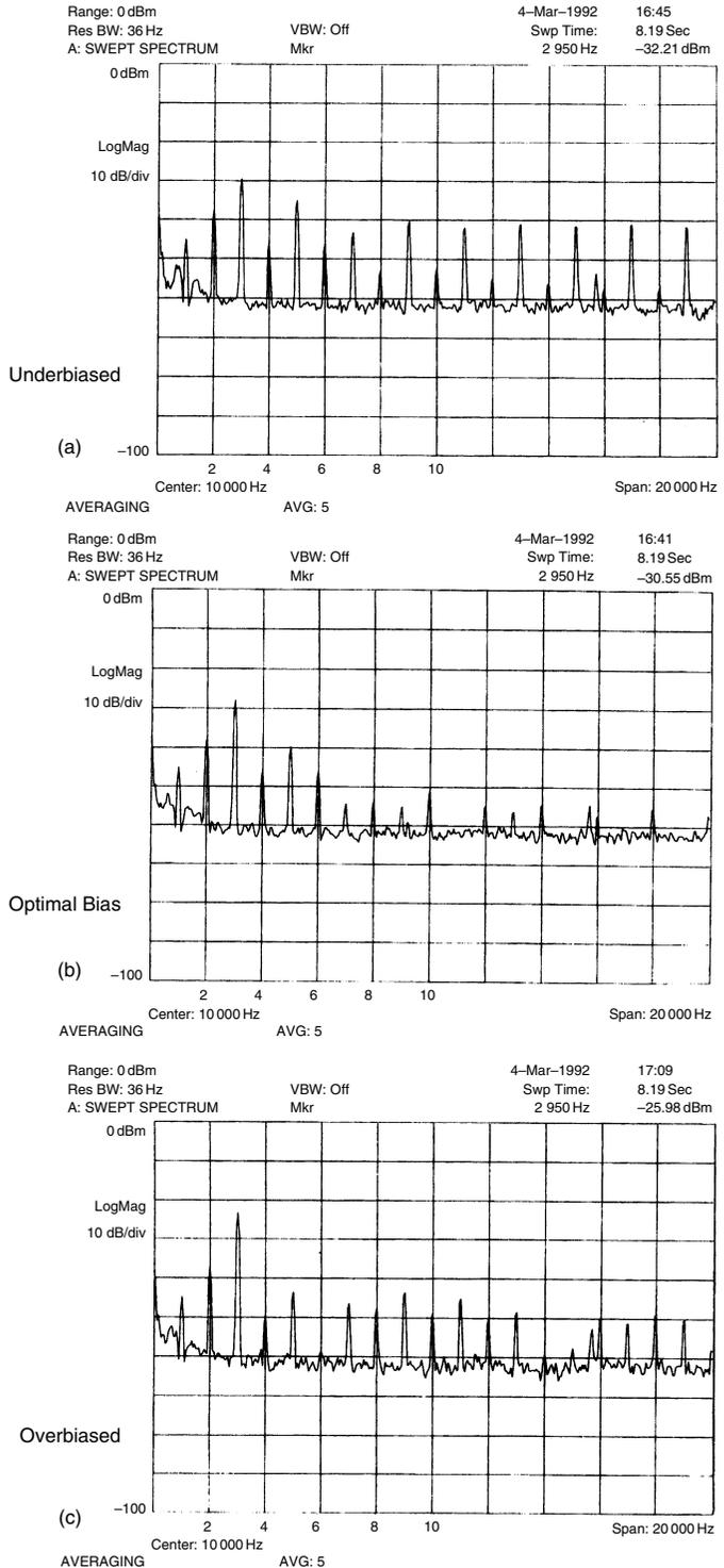
It must be emphasised that these effects are only visible in an amplifier where the other forms of distortion have been properly minimised. The RMS THD reading for Figure 5.1a was 0.00151%, for Figure 5.1b 0.00103%, and for Figure 5.1c 0.00153%. The tests were repeated at the 40 W power level with very similar results. The spike just below 16 kHz is interference from the testgear VDU.
