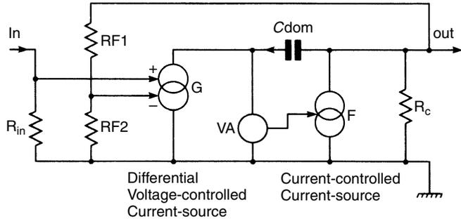
gain below the dominant-pole frequency P1 remains variable (and therefore so does P1) but is ultimately of little importance; if there is an adequate NFB factor for overall linearisation at HF then there are unlikely to be problems at LF, where the gain is highest. As for the input stage, the linearity of the VAS is not greatly affected by transistor type, given a reasonably high beta.
