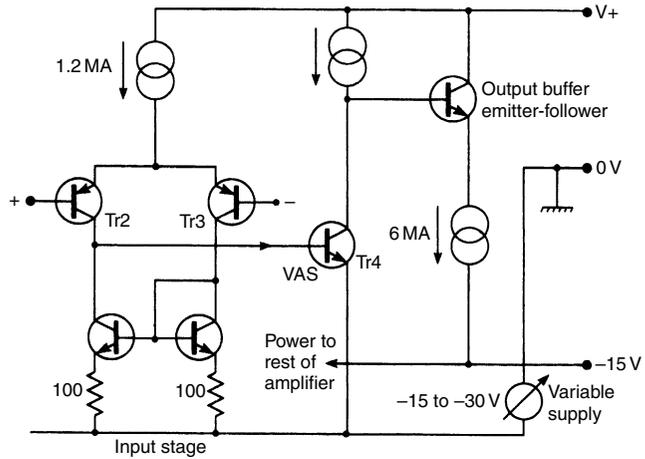
and down with the VAS emitter for correct operation, and so the  $V_{ce}$  of the input devices also varies, but this has no significant effect, as can be proved by the unchanged behaviour on inserting cascode stages in the input transistor collectors.
