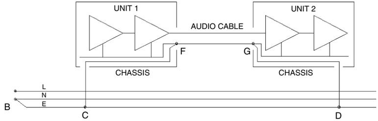
Balanced inputs will have no effect on this; they can cancel out the voltage drop along F–G, but if internal hum is introduced further down the internal signal path, there is nothing they can do about it.
