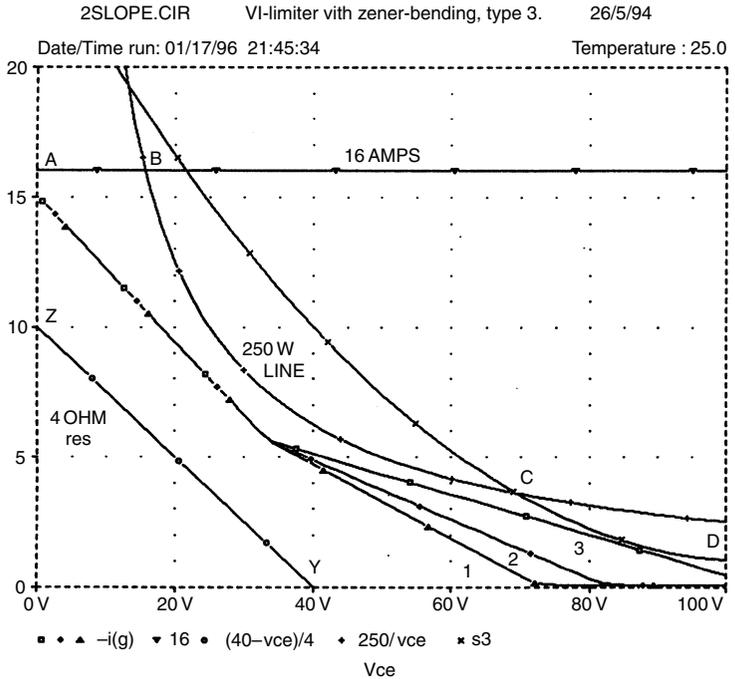
for Zener diode DZ1 to conduct. The series combination of R4 and R1 is chosen to give the required initial slope with low  $V_{ce}$  (i.e., the left-hand slope) but as the voltage increases the Zener conducts and diverts current through R5, whose value controls the right-hand slope of the protection locus. Loci 1, 2 and 3 are for  $R5 = 2\text{ k}\Omega$ ,  $1\text{ k}\Omega$  and  $1\text{ k}\Omega$ , respectively.
