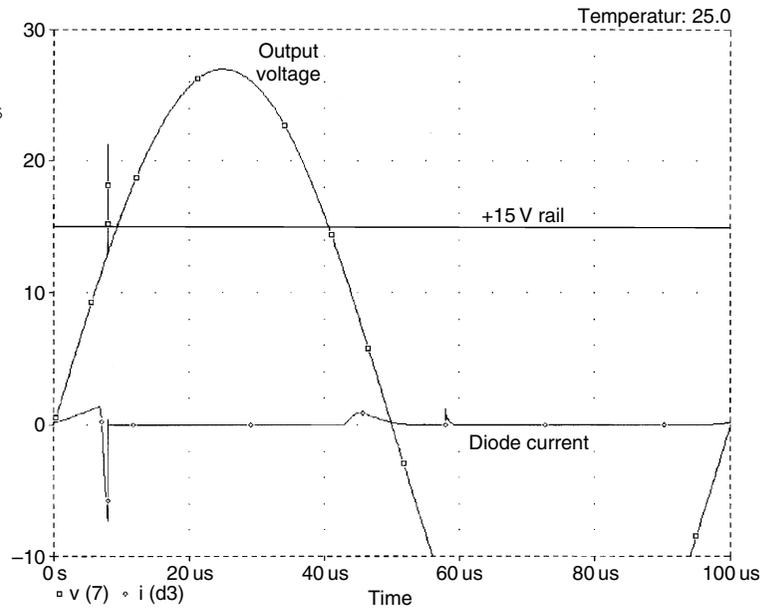
commutating diodes are Schottky rectifiers. Motorola MBR5025L diodes capable of 50 A and 25 PIV were used in simulation.
