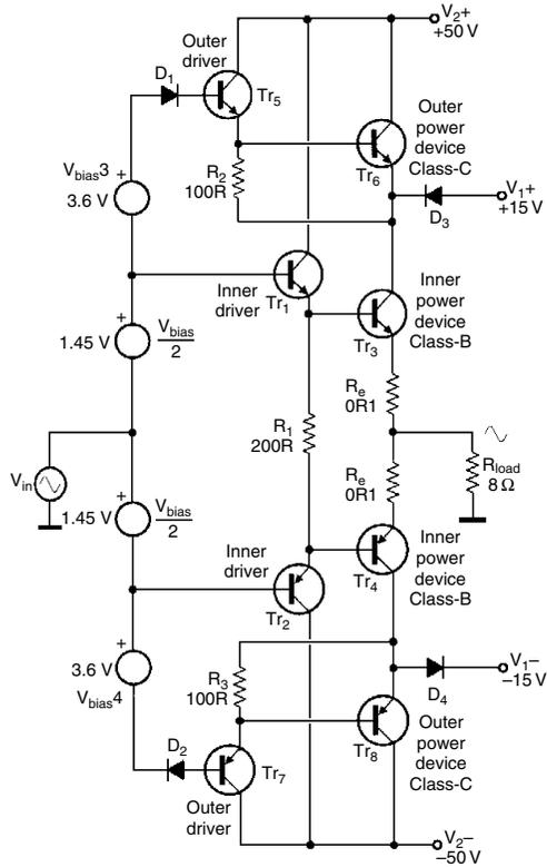
improvements made it is practical to proceed with the design of a Class-G amplifier with midband THD below 0.002%.
