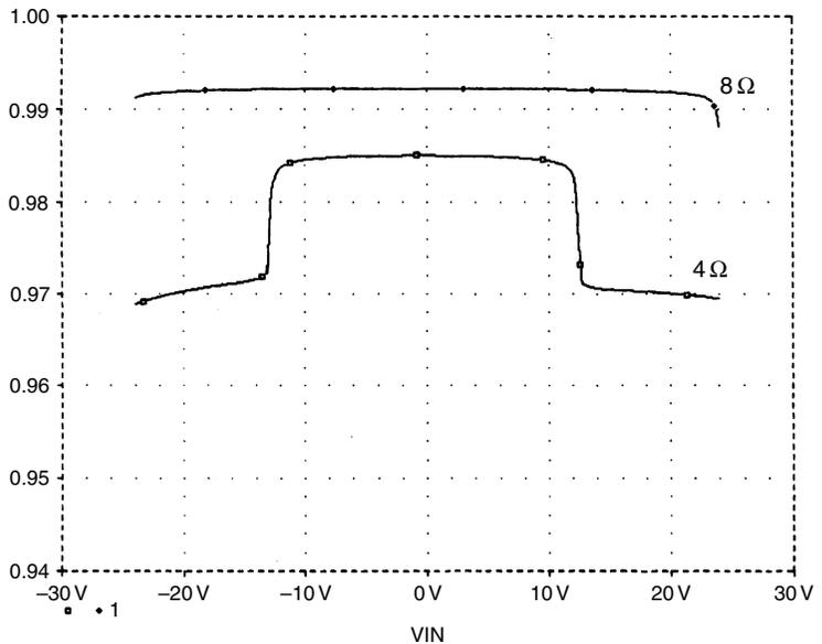
amplifier are shown in Figure 9.16, where it can be clearly seen that THD has been halved by this simple change. To the best of my knowledge this is a new result; if you must work in Class-AB, then keep the emitter resistors as low as possible, to minimise the gain changes.
