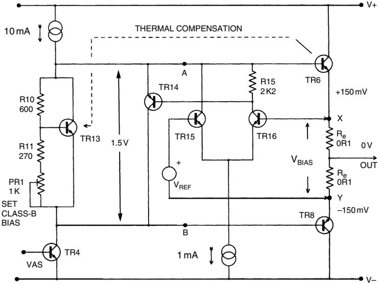
0.1  $\Omega$  emitter resistors, mainly by reducing the reference voltage to 300 mV, which gives a quiescent current ( $I_q$ ) of 1.5 A when established across the total emitter resistance of 0.2  $\Omega$ .
