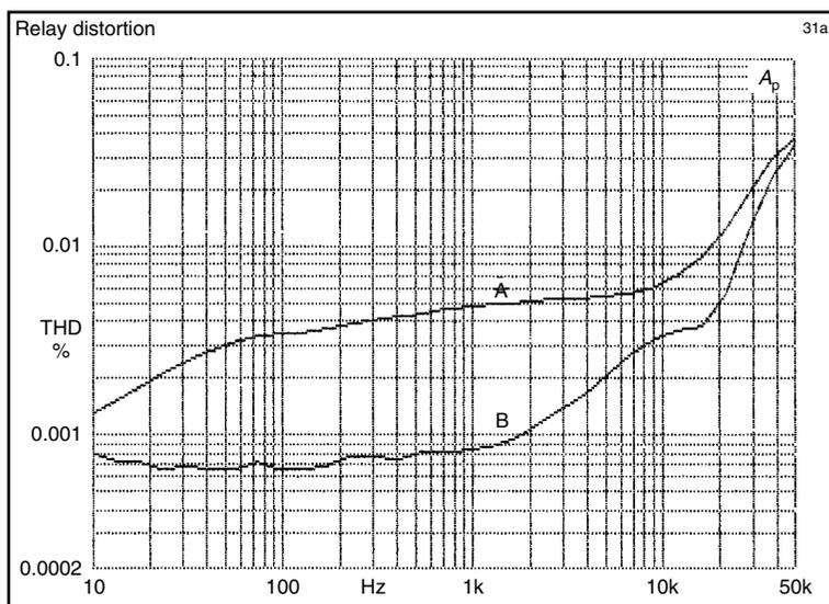
i.e., 10 Arms. Trace A is the raw extra distortion; this is lower than shown in Figure 15.21 because the same current is passing through less of the frame material. Trace B is the result of enclosing the frame fragment in the NFB loop exactly as before. This removes all suspicion of interaction with coil or contacts and proves it is the actual frame material itself that is non-linear.
