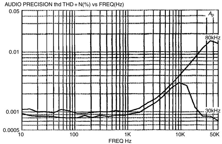
meaningless as all the harmonics are filtered out. All the Class-G plots here are taken at 80 kHz to make sure any high-order glitching is properly measured.
