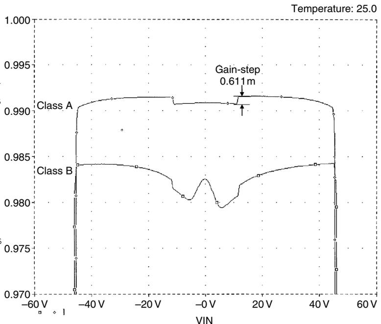
short order that the gain-steps were caused wholly by Early Effect acting on both inner drivers and inner output devices. The gain-steps are completely abolished. When TR6 begins to act, TR3 Vce is no longer decreasing as the output moves positive, but substantially constant as the emitter of Q6 moves upwards at the same rate as the emitter of Q3. This has the effect of a sudden change in gain, which naturally degrades the linearity.
