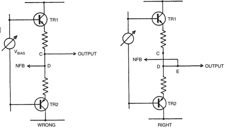
at output point C will have a half-wave rectified sinewave added to it, due to the resistance C–D. The actual output will be distorted but the feedback loop will do nothing about it as it does not know about the error.
