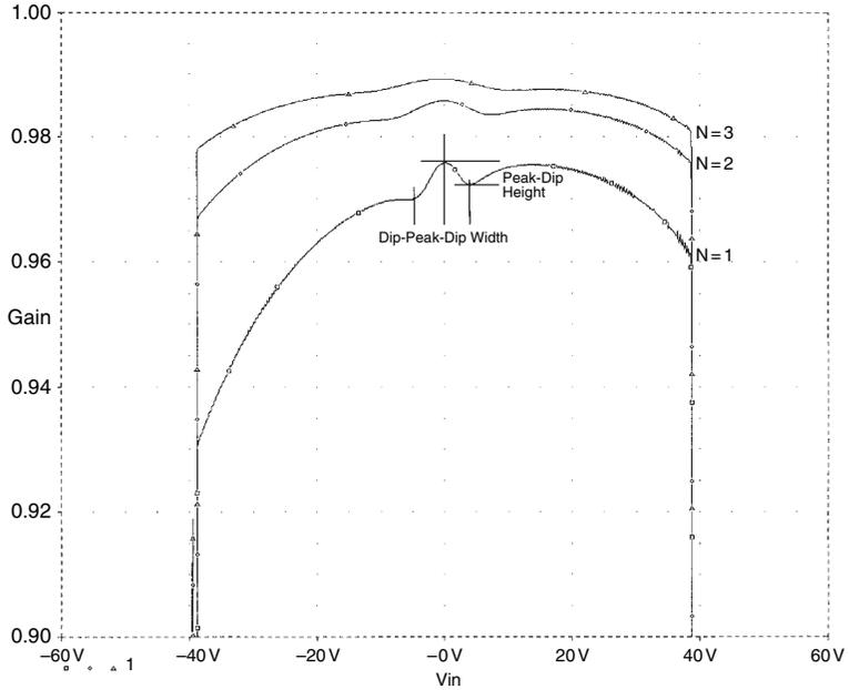
This makes sense. We know that crossover distortion increases with heavier loading, i.e., with greater currents flowing in the output devices, but under the same voltage conditions. It is therefore not surprising that reducing the device currents by using multiple devices has the same effect as
