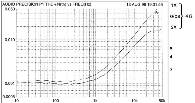
The output transistors used for this test were modern devices, the Motorola MJ15024/15025. The much older 2N3055/2955 complementary pair give a similar halving of LSN when their number is doubled, though the initial distortion is three times higher into 4 Ω. 2N3055 specimens with an H suffix show markedly worse linearity than those without.
