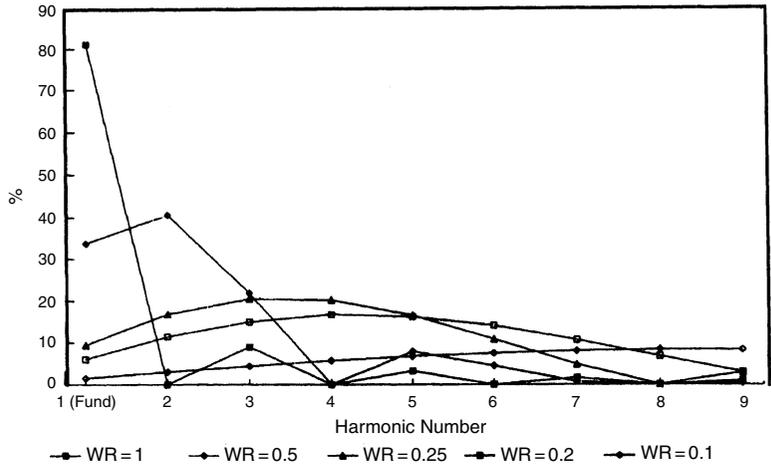
shows that most of the harmonic energy goes into the third and fifth harmonics; the even harmonics are all zero due to the symmetry of the waveform.
