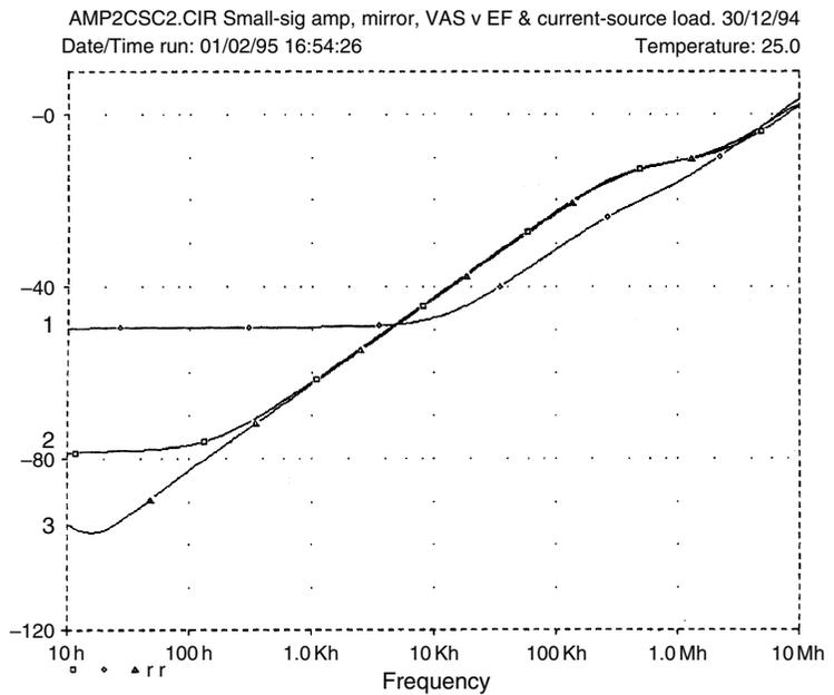
We still have a LF floor, though it is now at  $-80$  rather than  $-50$  dB. Extensive experimentation showed that this is getting in via the collector supply of TR12, the VAS beta-enhancer, modulating  $V_{ce}$  and adding a signal to the inner VAS loop by early effect once more. This is easily squished by decoupling TR12 collector to  $V-$ , and the LF floor drops to about  $-95$  dB, where I think we can leave it for the time being (Curve 3 in Figure 8.7).
