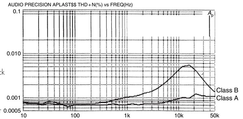
in Class-A for varying measurement bandwidths. The lower bandwidths misleadingly ignore the HF distortion, but give a much clearer view of the excellent linearity below 10 kHz. Figure 9.24 gives a direct comparison of Classes A and B. The HF rise for B is due to high-order crossover distortion being poorly linearised by negative feedback that falls with frequency.
