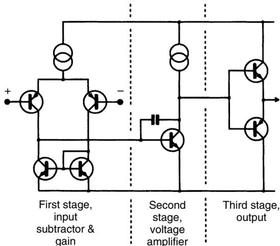
(virtual-earth) nature, and therefore very little on the first stage output; this minimises Miller phaseshift and possible Early effect in the input devices.
