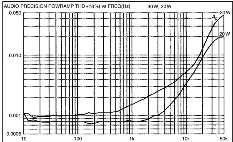
use of two-pole compensation can give you a Class-B amplifier that is hard to distinguish from Class-A – at least until you put your hand on the heatsink.
