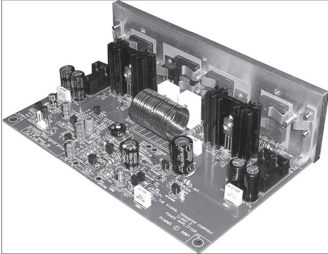
Shown above is the Class-G power amplifier, combining improved efficiency with first-class performance. The design is described in detail by Doug Self in Chapter 10.
