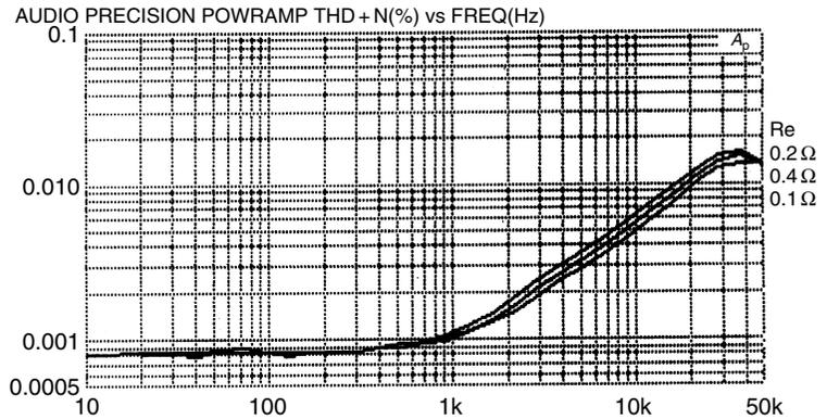
Having considered the linearity of Class-A and AB, we must not neglect what effect this radical  $R_e$  change has on Class-B linearity. The answer is, not very much; see Figure 9.17, where crossover distortion seems to be slightly higher with  $R_e = 0.2\ \Omega$  than for either  $0.1$  or  $0.4\ \Omega$ . Whether this is a consistent effect (for CFP stages anyway) remains to be seen.
