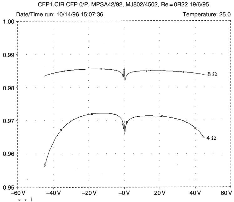
As it happens, an 8Ω nominal impedance is a reasonably good match for standard power BJTs, though 16Ω might be better for minimizing LSN if loudspeaker technology permits. It is coincidental that an 8Ω nominal impedance corresponds approximately with the heaviest load that can
