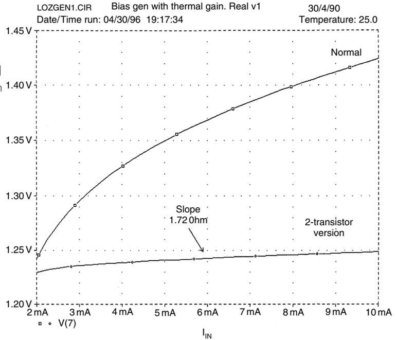
design of Class-B amplifiers with greater bias accuracy, and therefore less afflicted by crossover distortion.
