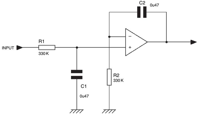
The component values shown in Figure 14.3 give unity gain at 1 Hz.
