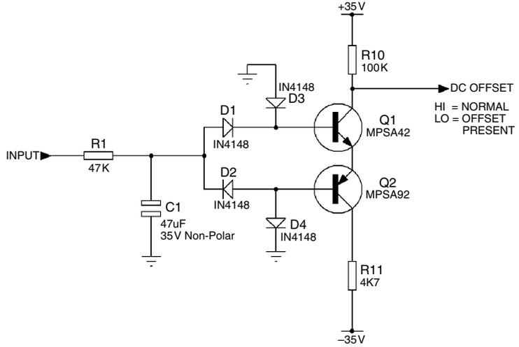
give thresholds of  $\pm 2.4\text{V}$ ; in practice the diode supplying the much smaller base current has a lesser voltage across it, and the real thresholds come to  $\pm 2.1\text{V}$ . Note that R11 is very definitely required to limit the current flowing through Q1, and Q2 when the input goes negative; R10 inherently limits it for positive inputs.
