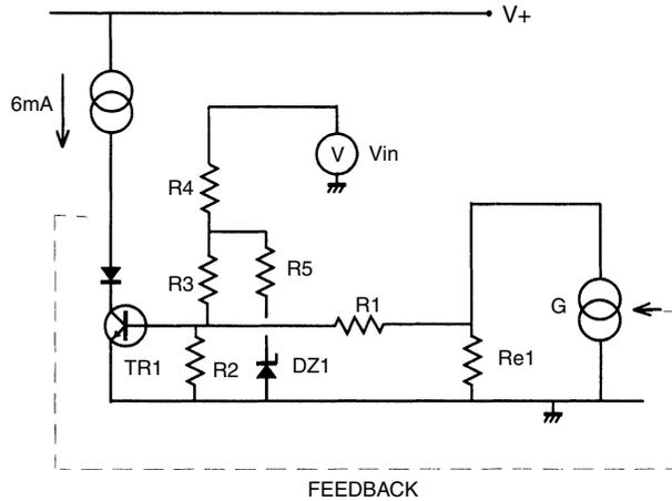
The feedback loop is closed by making the voltage at the collector of TR1 control the current flowing through G and hence Re1.
