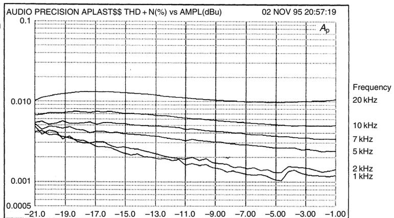
a selection of frequencies; Figure 5.40 shows the same for the CFP. Neither shows a significant rise in percentage THD with falling level, though it is noticeable that the EF gives a good deal less distortion at lower power levels around 1 W. This is an unexpected observation, and possibly a new one.
