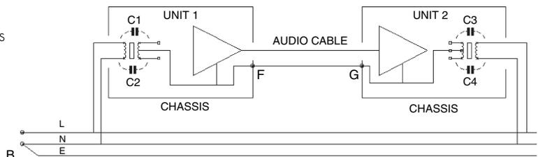
The magnitude of ground current varies with the details of transformer construction, and increases as the size of the transformer grows. Therefore the more power a unit draws, the larger the ground current it can sustain. This is why many systems are subjectively hum-free until the connection of a powered subwoofer, which is likely to have a larger transformer than other components of the system.
