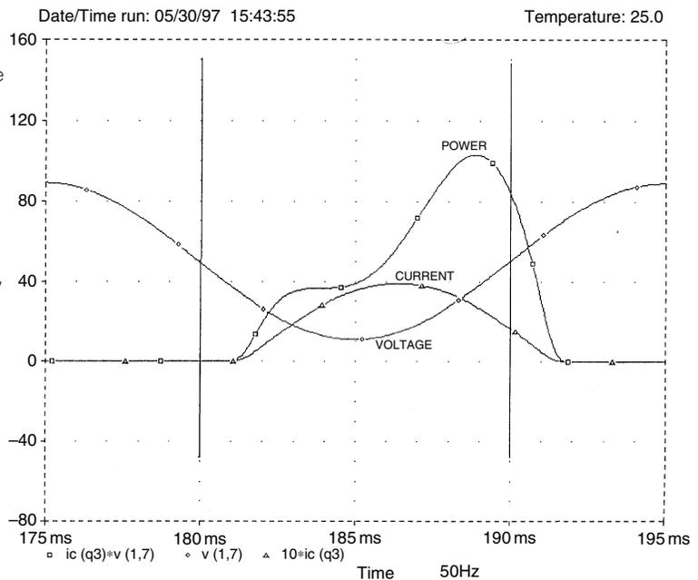
be considered at some point.) The critical quantities for semiconductor safety in amplifiers are usually the peak instantaneous values; for heatsink design average power is what counts, while for the power supply average current is the significant quantity.
