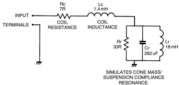
and air-spring of the enclosure, with  $R_r$  setting the damping; these last three components have no physical existence, but give the same impedance characteristics as the real resonance.
