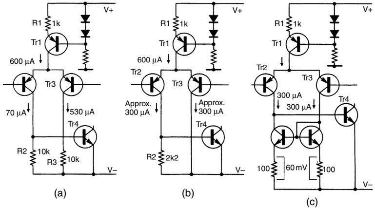
attempt to maximise o/l gain by minimising loading on Q1 collector. R3 is also 10k to give the stage a notional *balance*, though unhappily this is a visual rather than electrical balance. The asymmetry is shown in the resulting collector currents; the design generates a lot of avoidable second harmonic distortion, displayed in the 10k curve of Figure 4.8.
