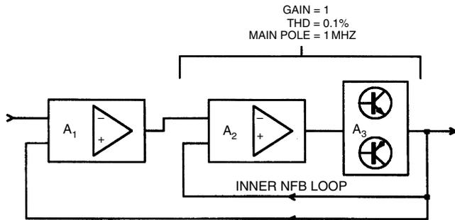
Miller loop around the second and third stages; global NFB is then applied externally around the whole lot. Nested Miller compensation has reached its apotheosis in CMOS op-amps – the present record appears<sup>[7]</sup> to be three nested Miller loops plus the global NFB; do not try this one at home. More details on the theory of nested feedback can be found in Scott and Spears<sup>[8]</sup>.
