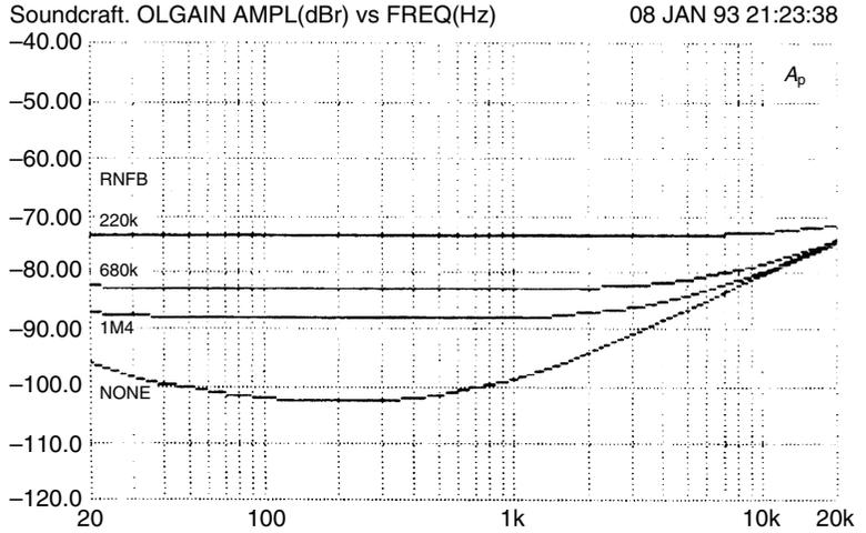
20 kHz by using a 220 k value for RNFB; however the gain at higher frequencies is unaffected and so is the stability. Although the amount of feedback available at 1 kHz has been decreased by nearly 20 dB, the distortion at +16 dBu output is only increased from less than 0.001 to 0.0013%; most of this reading is due to noise.
