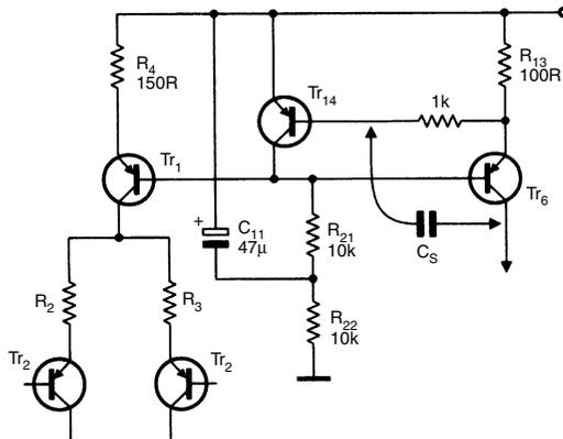
With  $R_4 = 100$ ,  $R_{13} = 68$  adding  $C_s = 6\text{pF}$  takes us from  $+37, -52$  to  $+42, -43$ ; and the slew asymmetry that has dogged this circuit from the start has been corrected. Fine adjustment of this capacitance is needful if good slew-symmetry is demanded.
