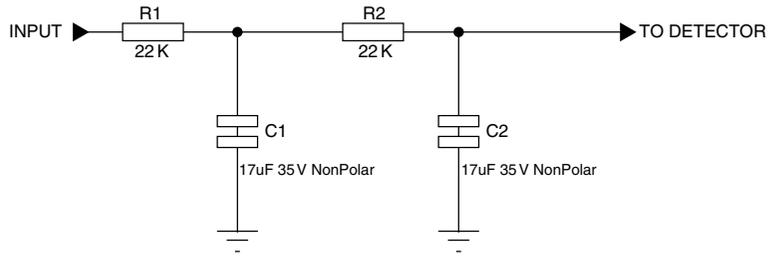
non-standard capacitor values shown give the same attenuation of  $-28.8$  dB at  $2.0$  Hz as the previous circuit. The only real snag to this scheme is that it does not work. The time to react was  $114$  msec, half as long again as the simple filter above. However I have seen it used in several designs, so you might come across it.
