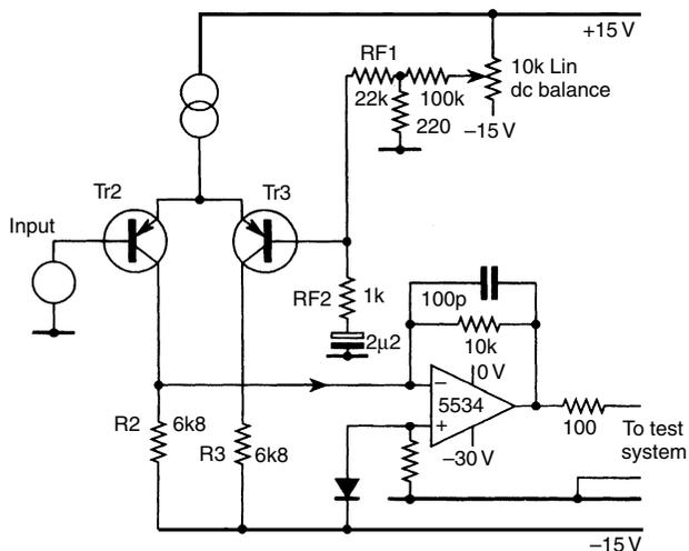
The differential pair has the great advantage that its transfer characteristic is mathematically highly predictable<sup>[2]</sup>. The output current is related to the differential input voltage  $V_{in}$  by:
