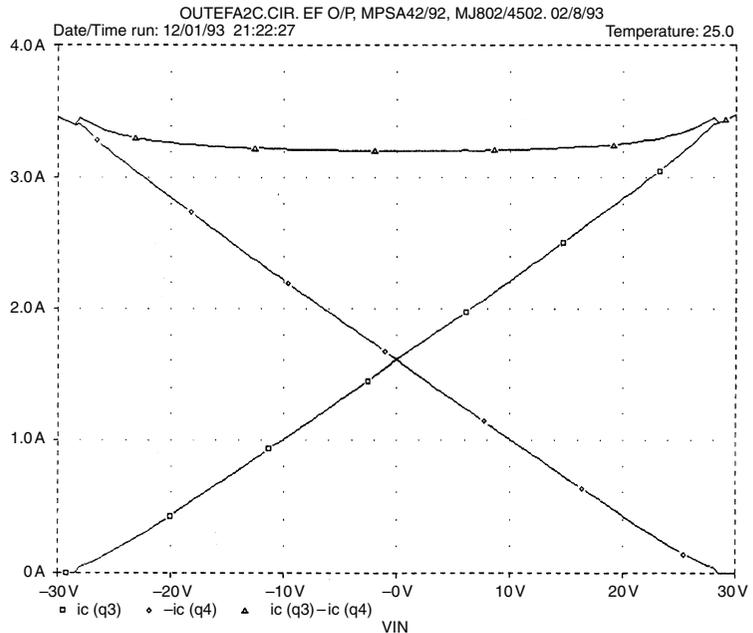
deviation from this constant-sum condition means increased inefficiency, as the stage must be conducting more current than it needs to for some part of the cycle.
