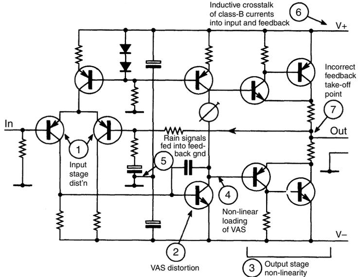
In Figure 3.2 an attempt has been made to show the distortion situation diagrammatically, indicating the location of each mechanism within the amplifier. Distortion 8 is not shown.
