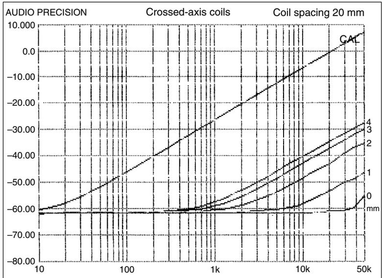
noise floor across the band, and a 2 mm misalignment now only worsens things by about 5 dB. This is definitely the best arrangement if the spacing is limited.
