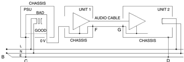
it directly reduces the fraction of the total loop voltage which is dropped between F and G.
