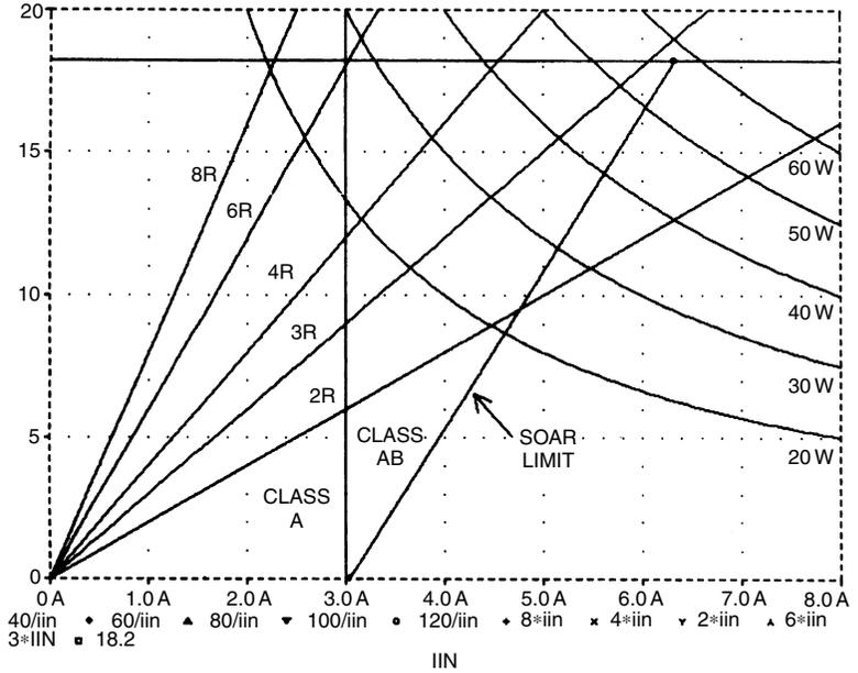
sloping up from the origin and the ultimate limits of voltage-clip and SOAR protection define which of the curved constant-power lines is reached.
