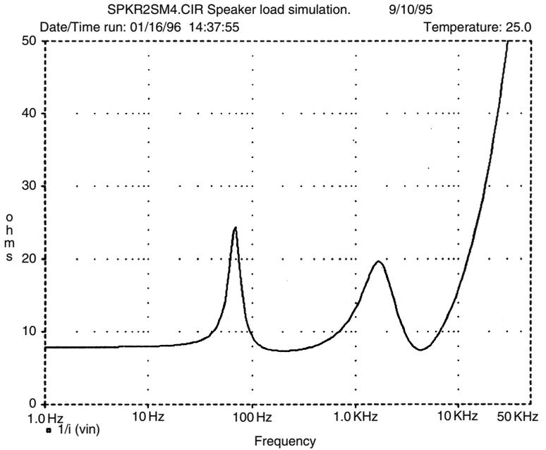
low-frequency unit, and this adds several extra variables to the situation. In a bass reflex design the bass resonance hump may be supplemented by another LF resonant peak due to the port tuning. An attempt at a representative load simulator for a two-way infinite-baffle loudspeaker system is shown in Figure 7.30. This assumes a simple crossover network without compensation for rising tweeter coil impedance, and is partially based on a network proposed by Ken Kantnor in Atkinson<sup>[1]</sup>.
