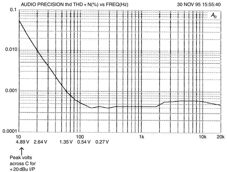
a 680Ω load, while Figure 6.15 shows how the associated LF roll-off has barely begun. The distortion is a mixture of second and third harmonic, and rises rapidly as frequency falls, at something between 12 and 18 dB/octave.
