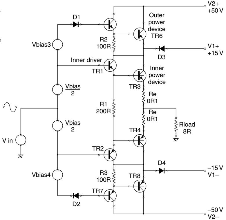
To the best of my knowledge three-level Class-G amplifiers have only been made in Shunt mode, as described below, probably because in Series mode the cumulative voltage drops become too great and compromise the efficiency gains. The extra complexity is significant, as there are now six supply rails and at least six power devices all of which must carry the full output current. It seems most unlikely that this further reduction in power consumption could ever be worthwhile for domestic hi-fi.
