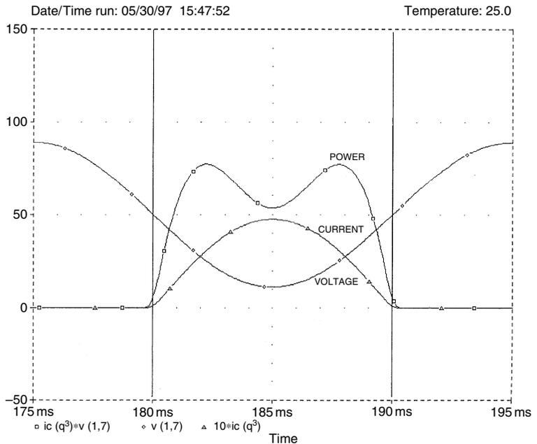
characteristic two-horned shape, peaking twice at 77 W during its conducting half-cycle.
