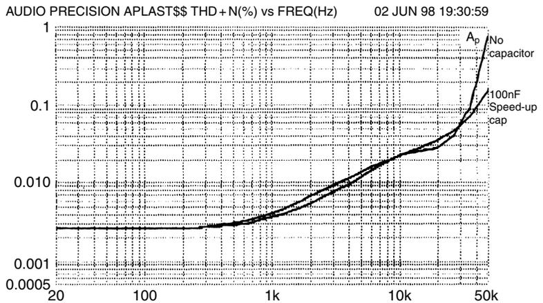
Figure 5.46 shows the reduction of HF THD by adding a speedup capacitor across the common driver resistor of an EF Type II. At LF the difference is small, but at 40 kHz THD is halved, indicating much cleaner switchoff. There is also a small benefit over the range 300 Hz–8 kHz.
