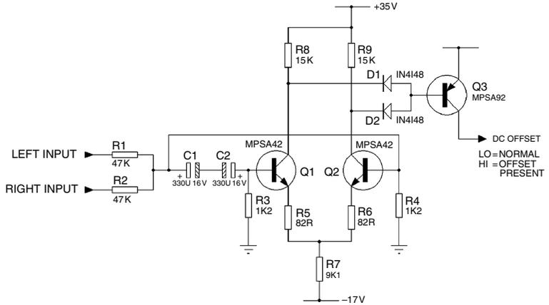
VLF information. The result is then subtracted from the unfiltered signal by the differential pair, so only the DC and low frequency signals remain.
