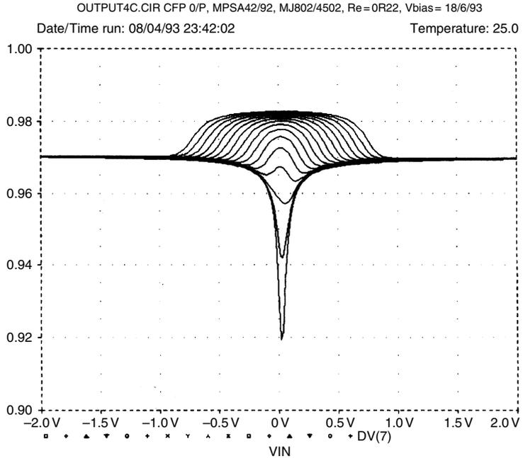
The crossover region is much narrower, at about  $\pm 0.3\text{ V}$  (Figure 5.10). When under-biased, this shows up on the distortion residual as narrower spikes than an emitter-follower output gives. The bad effects of gm-doubling as  $V_{\text{bias}}$  increases above optimal (here  $1.296\text{ V}$ ) can be seen in the slopes moving outwards from the centre.
